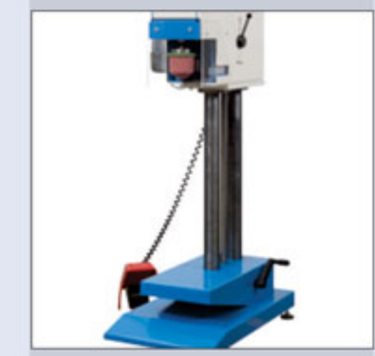
^ Machine table with very large adjustment track
