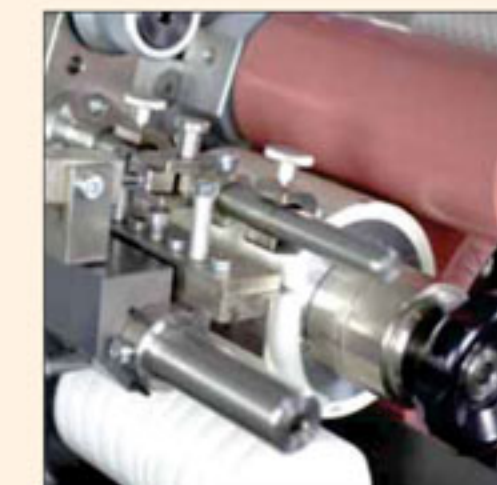
▲ "H-RTI 21-150" with Ø 100 mm ceramic cliché cylinder and 50 mm spacer
