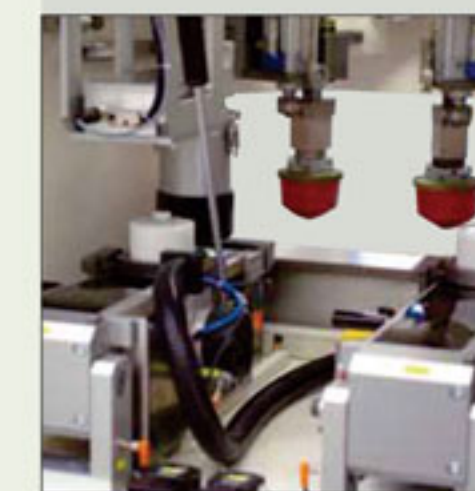
^ 2 printing stations equipped with "microflex" cliché band
