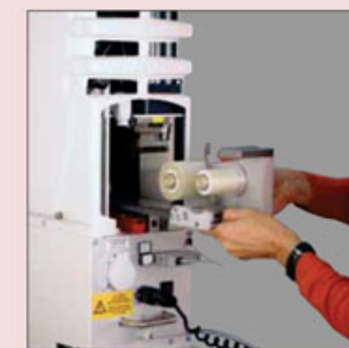
^ Ink residue pick-up system (pad cleaning)
