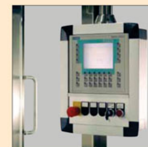
^ Control of the Modul automations via touch screen
