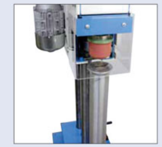
^ Example for utilization of the large working area: Printing on the face of a cylinder
