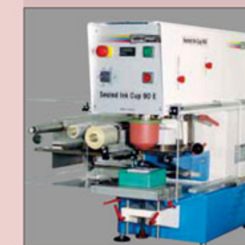
^ With fitted ink residue pick-up system
