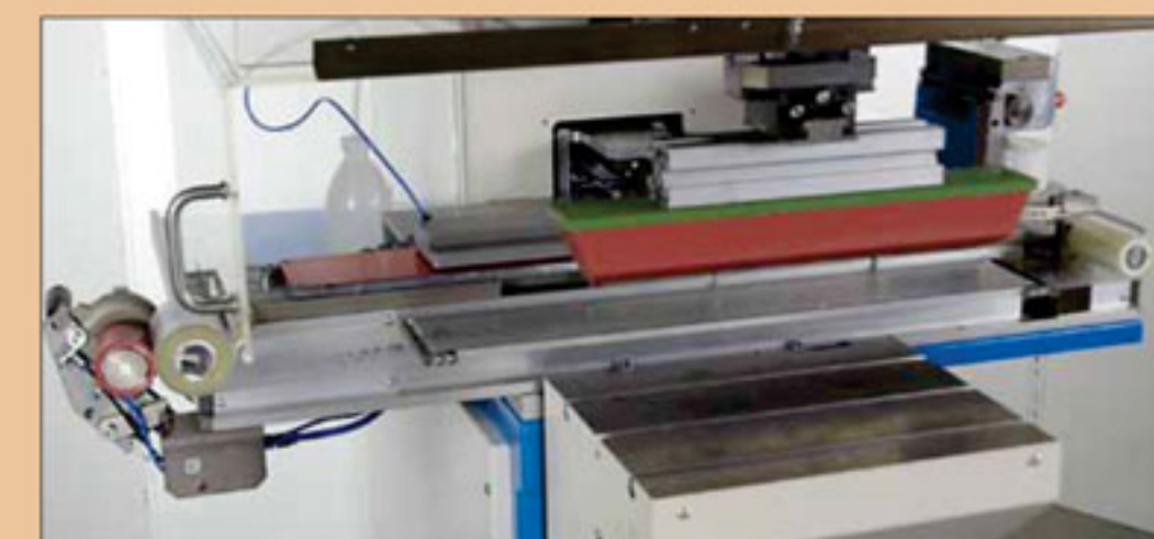
▲ "TSM 60/90" with "hermetic" transverse doctor blade kit - replaces our TSQ series
