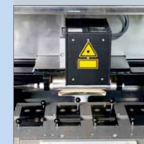
Linear motor axis with receiver plate for 4-colour screen set
